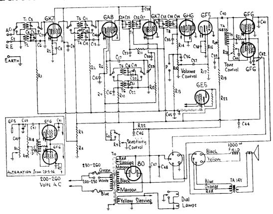
abiloLA models "251" and "303" use chasses of identical design, the difference between the two models being found in the cabinet style and the fact that model "303" is equipped as a "radiogram" by the incorporation of a pick-up, motor, and automatic record-changing device. The basic model, however, is the "251" and this will be described.
